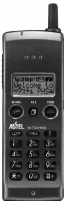
Photo 1. ASTEL's PHS terminal — the world's smallest handset as of May 1997 (weight: 80 g; volume: 66 cc; call duration time: 5 hours; standby time: 450 hours)
